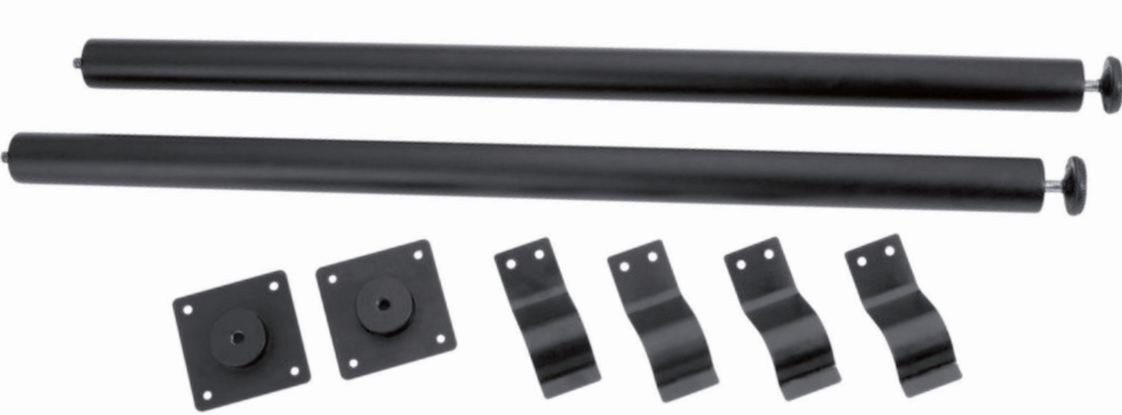
87990 RACK TABLE LEGS 75 - 78 CM 2-Leg system with steel mounting plates, incl. holding clamps to mount inside case lid. Length: adjustable from 75 cm to 78 cm. Leg with 30 mm height adjustment. M10 thread on leg and foot. Colour: black powder coated
