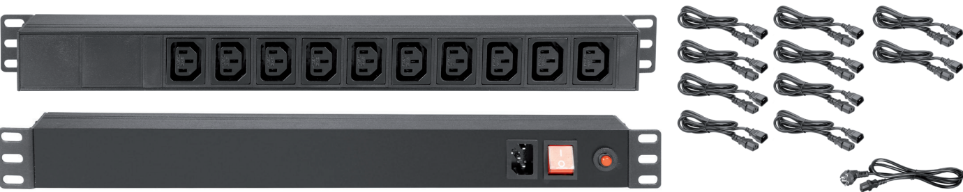
87471IEC 19" POWER STRIP 1 U WITH 10 IEC CONNECTORS This 1U rackmount power strip provides ten IEC C13 grounded outlets on the rear of a 19" aluminum enclosure. The front panel features a C14 male inlet, an illuminating master on/off switch and a resettable circuit breaker for overload protection
