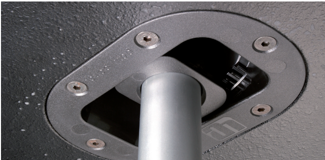
SM707 ANGLE SPEAKER TOP HAT Adjustable Angle Speaker Top Hat for Loudspeaker incl. gasket. Vertical angle can be adjusted in 4° increments to +/- 18°. Fits SPS56B and most other standard speaker stands. Internal ø 36 mm. Black Polyamide. Maximum Load 40 kg. Patented.
