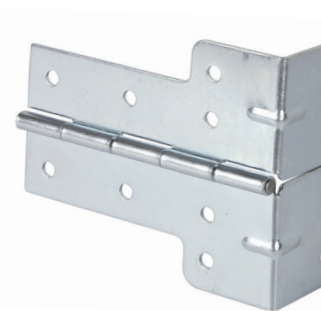
2641 L-HINGE LARGE L-hinge large. Similar to 2640 , but a combination of corner brace 40403 and piano hinge 2606 . Steel, 1.5mm, zinc plated, fixing holes ø 5.1mm.
