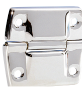
2508 MEDIUM STOP HINGE Stops at 95° Steel, chrome plated Thickness 1.0 mm Fixing holes ø 4.1 mm Weight 26 g
