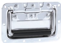
34082 RECESSED SPRUNG HANDLE In 8 mm deep dish with black PVC grip. Fixing holes ø 5.1 mm, weight 360 g.
