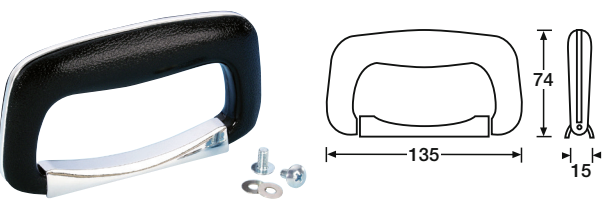
3438 BRIEFCASE DROP HANDLE Quality Briefcase drop handle. Solid black plastic grip with chrome decorative insert. Fixing plate chrome plated diecast. Fixings M5 x 10 mm (supplied), weight 100 g.
