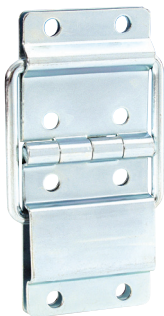
2524 / 2524CHR STRUT HINGE Extra heavy duty strut hinge with backplate. Steel, zinc or chrome plated Strut \varnothing 4.0 mm Fixing holes \varnothing 5.1 mm Weight 80 g
