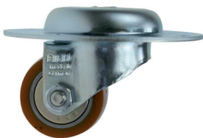
37041 SWIVEL CASTOR WITH HEAVY DUTY WHEEL The main features of this swivel castor are high stability, low height and excellent steering ability. This heavy duty ball bearing castor has a loading capacity of 100 kg. It has a low noise level and is abrasion-proof. This castor is mounted on a 10 mm deep, galvanized steel fitting. The overall height after mounting is thus only 41 mm, weight 300 g.
