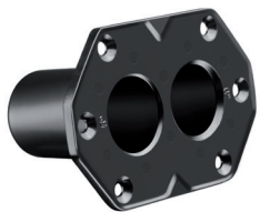
SM7DT DUAL-TILT FLANGE (0°/5°) Mounting flange with 0° and 5° horizontal tilt for loudspeaker cabinets on speaker stands, inner diameter 36 mm, depth 76 mm. Weight 375 g.
