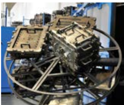
Pictured: Molds rotating during production.
