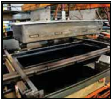
Pictured: Vacuum mold for keyboard case.
