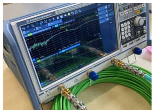
12G Measuring station at the KLOTZ factory in Vilchband
